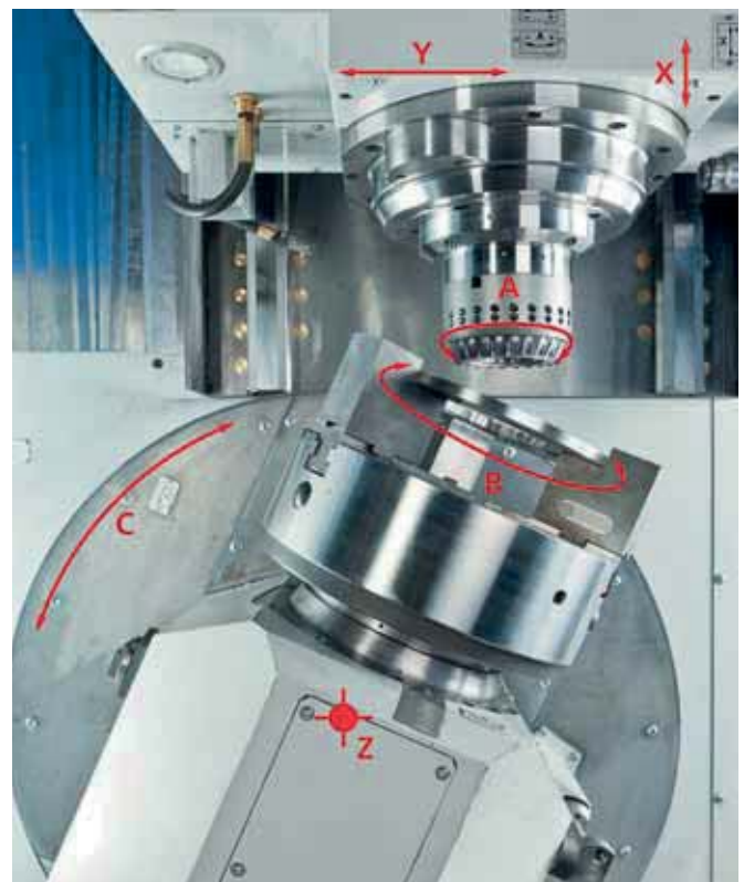
Fig. 5: Skiving on an Oerlikon Spiral Bevel Gear Cutting Machine C 29 – the machine axes are shown in red.
