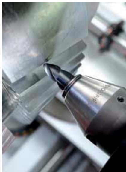
Fig. 5: Roughing and tooth root machining
