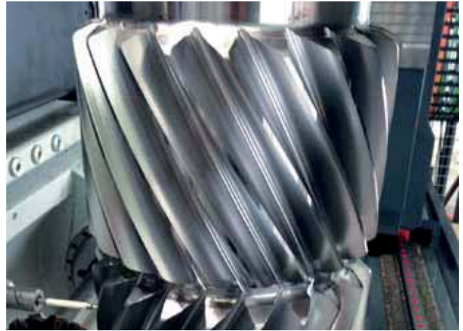
Example component, shaft (m8.8; d_a=271 mm)
