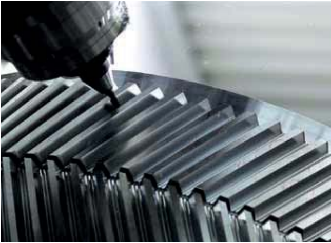
Example component, gear (m8.8; d_a=1023 mm)
