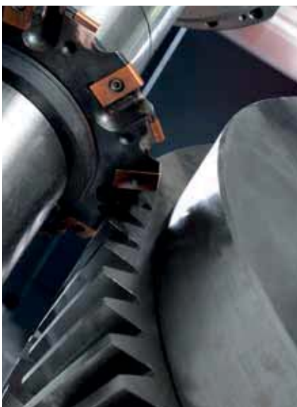
Fig. 4: Maximum productivity benefits thanks to pre-machining with form milling tools
